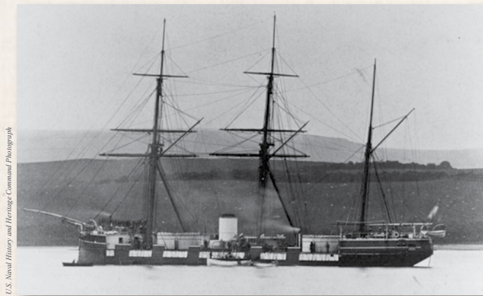
The Wivern was one of two ironclads built for the Confederacy by the Laird Company in Great Britain but never delivered because of U.S. diplomatic protests. The working plans for the Laird ships included twin gun turrets, 4.5 inch-thick iron plating, and a bow reinforced with wrought iron for ramming enemy ships.
